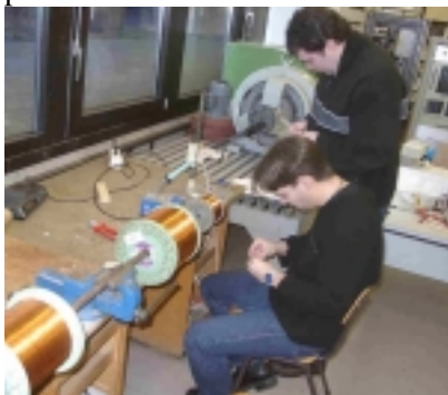
Figure 8 Students are winding transformer-coils
